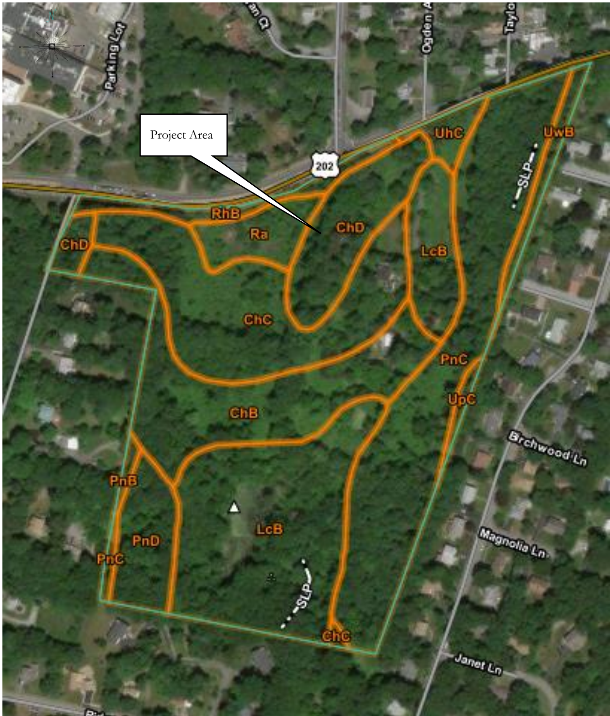
Figure 2: Aerial Image showing soil units within the Project Area. (Source: Natural Resources Conservation Service.) Scale: 1"=200'.
